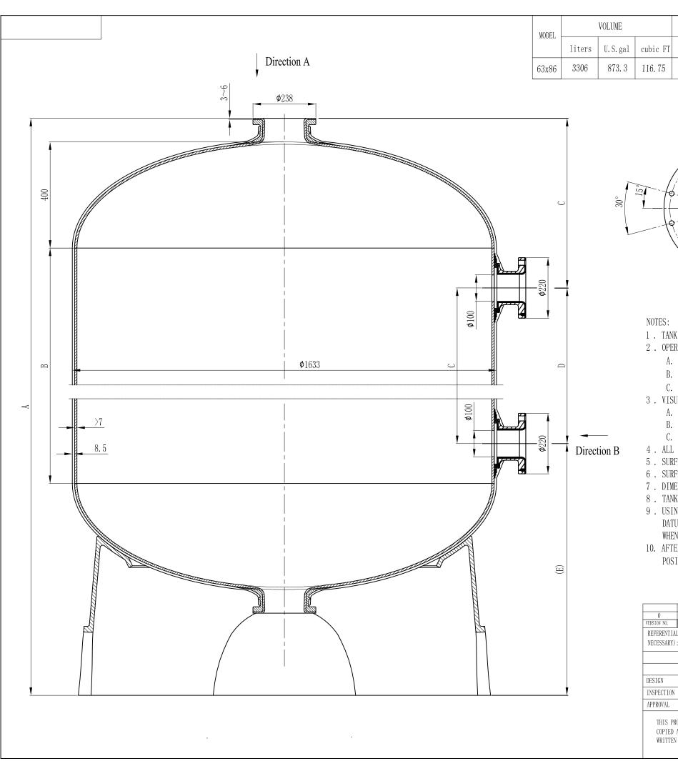
DOME VOLUME WEIGHT B (mm) D (mm) (E) (mm) A (mm) C(mm)liters | U.S.gal LBS cubic FT Kg 135.0 660 816 999 511 18.06  $367.7 \mid 810.6 \mid 2475 \pm 15 \mid 1158$
